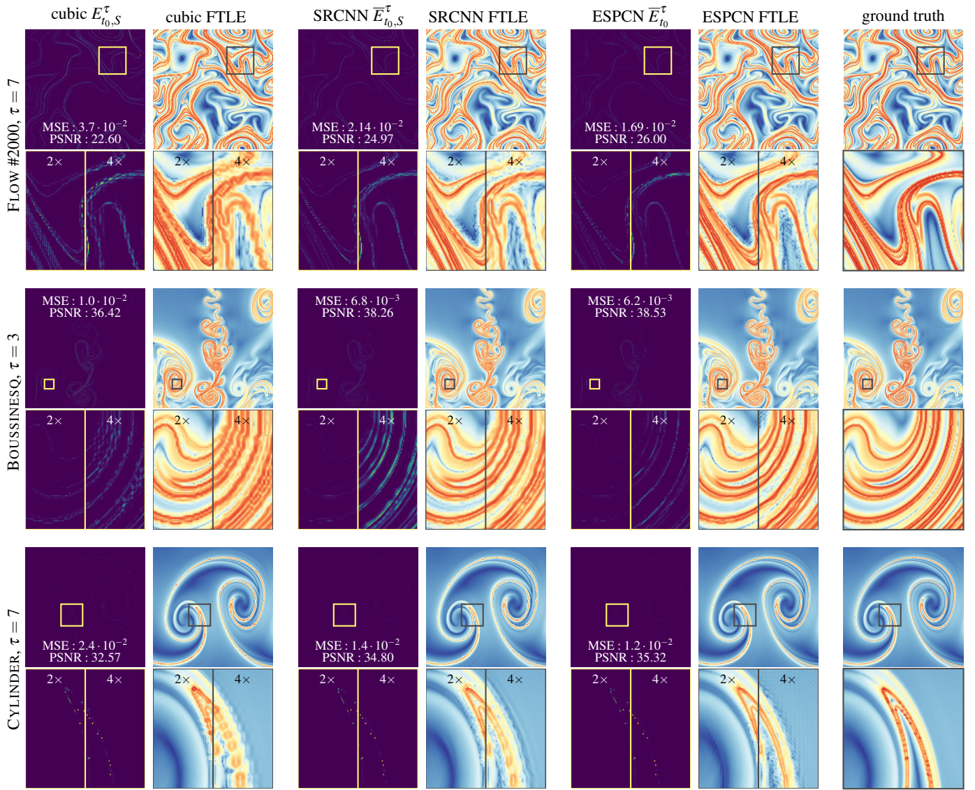
Fig. 10: Error maps and FTLE comparisons for different fluid flows. In all cases, the flow map was traced from t_0 = 0 up to \tau . The top row of each data set contains the overview of the 2\times upsampling and the quantitative error measures. The close-ups compare the 2\times and 4\times upsampling.
