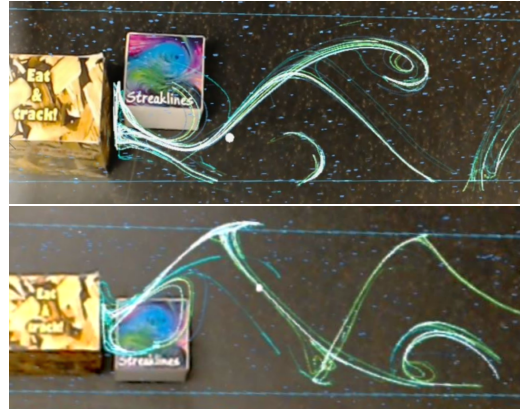
Figure 4: Flow visualizations, showing the impact of different inflow velocities on the vortex patterns. Top: slow inflow velocity, bottom: fast inflow velocity.
