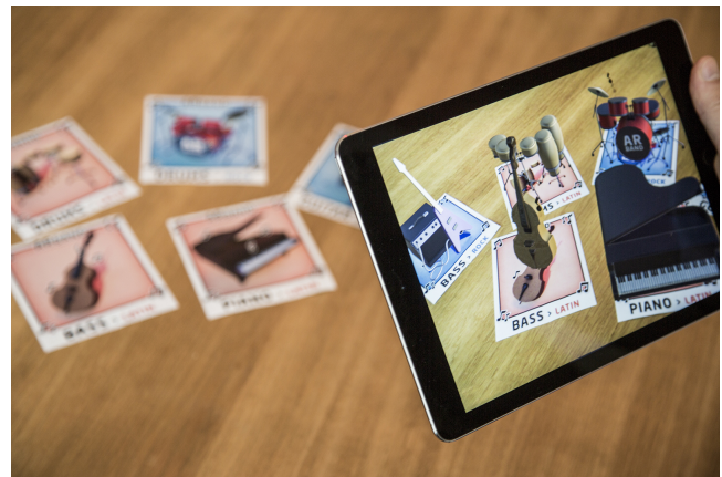
Figure 7: The user listens to the arrangement he or she just created using the markers on the table while observing the virtual instruments on the iPad.
