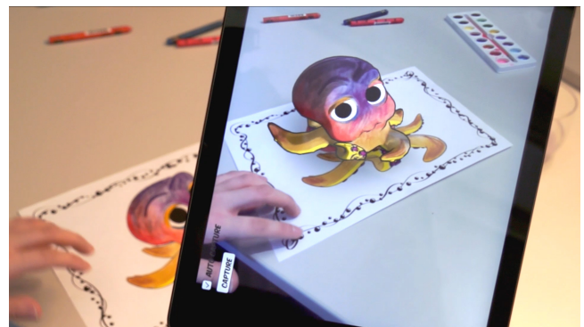
Figure 3: After coloring the octopus character, the user inspects the automatically textured 3-D model of the octopus on the iPad.
