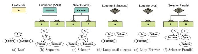
Figure 4: Control flow graphs for the different control nodes used in Behavior Trees.
