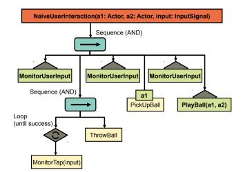
Figure 2: Handling user interaction in a traditional Behavior Tree. The MonitorUserInput subtree is required at all points in the narrative tree where the user selects how the narrative proceeds, resulting in unnecessary large trees.
