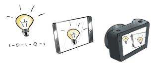
**Figure 5:** Latency measuring setup. The mobile device running ARTravelers is pointed at blinking LEDs. A high-speed camera captures both, the LEDs and the LEDs on the display. The recorded video can then be analyzed to calculate the delay between the LEDs and the LEDs on the display.
