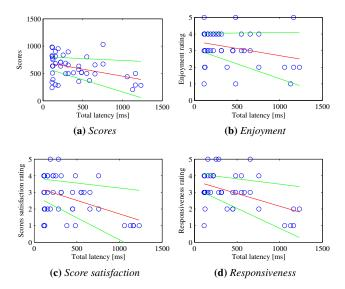
**Figure 8:** Linear regressions of scores, enjoyment, scores satisfaction and responsiveness over total latency. The red lines depict the fitted linear curves and the green lines define the lower and upper limit of the 95% confidence interval.
