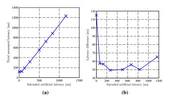
**Figure 7:** (a) depicts the total measured latency over the intended AAL. (b) shows the native latency (i.e. the difference between the total measured latency and the intended AAL) over the intended AAL
