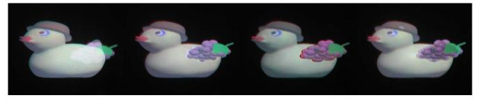
Figure 1: Illustration of the steps of our light field decomposition. (1) volumetric rendering, (2) view-independent and (3) viewdependent occlusion culling, (4) view-dependent rendering on parallax type layer. Photographs are taken from our multilayered display prototype.
