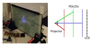
**Figure 7:** Our physical prototype consists of three emissive layers and a front most modulating layer.
