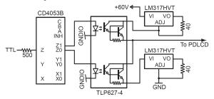
**Figure 6:** Circuitry used to create an alternating square wave function to drive the PDLC layers.
