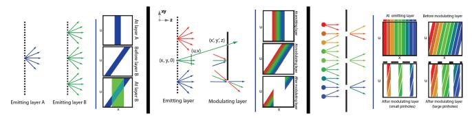
**Figure 2:** The three basic display layer primitives. Overlay of two emissive layers is shown on the left, impact of a modulating layer in the middle and the principle of a parallax barrier layer on the right.
