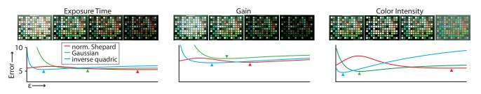
Figure 4. Average reconstruction error of the considered basis functions while interpolating 50% of the color checker fields under changing camera parameters. The error is shown as a function of the  $\epsilon$ -values for the normalized Shepard (red), the Gaussian (green), and the inverse quadric (blue) basis functions. The plots show that the  $\epsilon$  value significantly influences the result.
