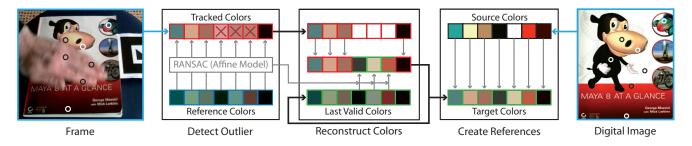
Figure 6. Overview of our stable color tracking pipeline. First, color values are extracted from the video frame and corrupt ones are rejected using RANSAC and temporal coherence. Then, missing colors are added using information from the previous frames. Finally, the stable color list is combined with colors from a digital image to create the transfer constraints that can be used for balanced augmentation of rendered objects.
