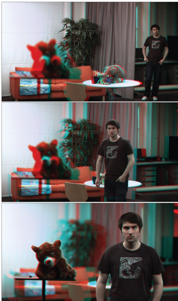
Figure 3: Example of automatic subject tracking for follow focus and convergence. Manual interaction is only required in the first frame (top), to initialize the subject of interest. In the following frames, our controller keeps the convergence plane and focus at the depth of the subject
