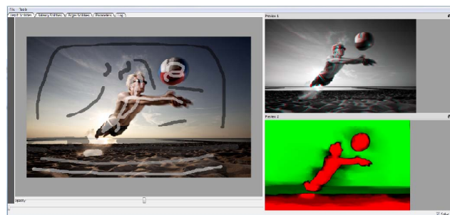
Figure 11: This is a screenshot of our StereoBrush application, showing user scribbles and two real-time visualizations of scene depth
