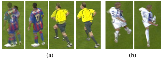
Figure 10: (a) Direct comparison for a view in the middle of two source cameras. Each player is rendered with a standard billboard technique and with articulated billboards. The standard billboards exhibit considerably ghosting artifacts. (b) An example of a bird's eye perspective. While standard billboards are simply tilted (left), articulated billboards give an impression of the actual 3D pose.
