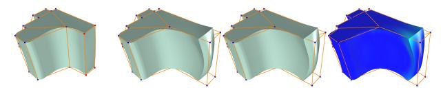
Fig. 2. From left to right: (a) The fan model is deformed by pulling the four red control points. (b) Shading using the exact normals. (c) Shading using the approximate normals. (d) Color plot of the approximate normals deviation (maximum deviation is 23 degrees, mean deviation computed only for the modified fine scale vertices is 1 degree).
