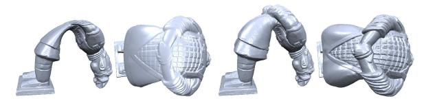
Fig. 6. The original *free-form* space deformation approach of Botsch and Kobbelt does not preserve fine surface details under large deformations (*left*). Integrating this technique into our GPU-based two-scale multiresolution framework yields much better results at almost the same speed (*right*). Even for this extreme deformation the average error of our approximate normal reconstruction is only 5 degrees.
