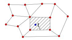
Fig. 4. Catmull-Clark surfaces basis functions' support: only the basis functions associated with the control vertices (red dots) incident to a face adjacent to the marked patch do not vanish for any parameter value  $t_i$  in the center face.
