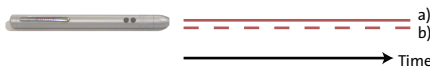
Figure 11: Mouse navigation using dual mode laser modulation: a) Pointing operation. b) Triggering operation.
