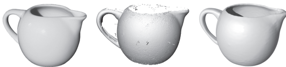
Figure 14: Reconstructed coffee creamer, from left to right: Physical model, acquired data set, reconstructed model.
