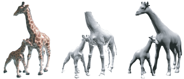
Figure 15: Shape reconstruction from low-quality data, from left to right: Physical model, acquired data set, reconstructed model.
