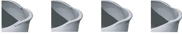
Figure 13: Stitching, from left to right: Initial configuration, two intermediate steps of alignment, final stitched model.
