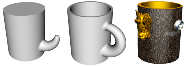
Figure 17: Creating the Siggraph coffee mug using boolean operations, deformation, collision detection and particle-based blending (see Figure 1 (c)).
