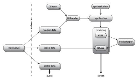
**Figure 3:** Dataflow of a typical JAPE application.
