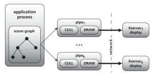
Figure 2: The multi-head rendering concept.
