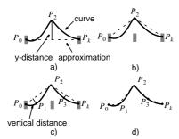
**Figure 12:** a) Recursive algorithm assuming a smooth representation of the underlying curve: a)  $P_2$  has largest vertical distance. b) new approximation after insertion of  $P_2$ . c) example for vertical distance measure. d) final result.
