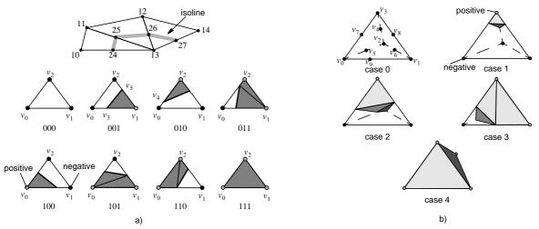
**Figure 16:** Polyline approximation of isolines: a) Isoline as computed by intersections with the triangle edges and look-up table to extract interior or exterior parts of the surface. b) Generation of isosurfaces and interior volumes using a marching tetrahedron algorithm: 5 basis cases arising upon triangulation. The connectivity table for generation of interior volumes is presented in Table 3.
