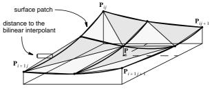
**Figure 13:** Extension towards multiple dimensions exemplified for nonparametric data: 2D version. The underlying B–spline patch is outlined in bold. A new vertex is inserted at position **P** and the distance is computed with respect to the bilinear-interpolant of  $\mathbf{P}_{ij}$ ,  $\mathbf{P}_{ij+1}$ ,  $\mathbf{P}_{i+1jr}$ ,  $\mathbf{P}_{i+1jr+1}$ .
