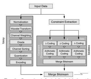
**Figure 6:** Compression pipeline including both lossless and lossy data compression. For decompression, all of the above steps have to be reversed.
